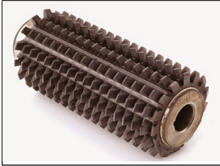
Fig. 5. Illustration of a generic hob.
